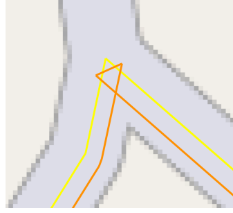
(b) Wrong offset - offsetting and drawing both start and end coordinates of each line. Yellow - original polyline, orange - offset polyline.
